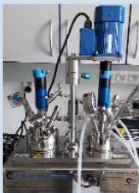
High pressure batch reactor
