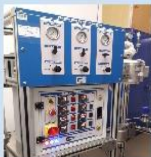
High pressure flow reactor
