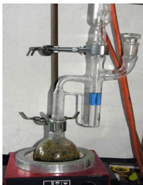
Fig.2.: Apparatus for the preparation and isolation of chamazulene from chamomile essential oil
