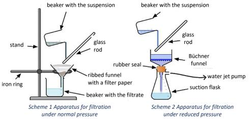
Equipment: beakers (150, 250, 400 ml), watch glass, graduated cylinder (100 ml), water jet pump, Büchner funnel, suction flask, ribbed funnel, iron ring, filter paper, scissors, glass rod, spatula, crystallising dish
