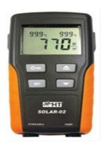
PURPOSE: The remote unit SOLAR-02 has been designed to measure sun irradiation (W/m²) and temperature (°C) by means of appropriate probes connected to it. It can also be used in combination with an HT Italia instrument with USB connection (SOLAR300, SOLAR300N) and with RF connection (SOLAR I-V, I-V, I-V400) to carry out the above-mentioned measurements for testing/recording the efficiency of single-phase and three-phase photovoltaic installations and detection of I-V curve of PV module/strings.
